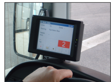
Automated displays linked to GPS keep drivers on track and on time.
